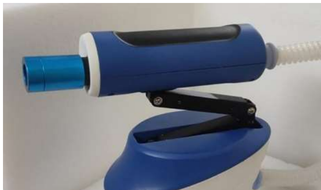
Figure 16 Reference Impedance connected to FOT tube
